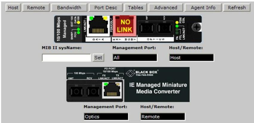
A navigation bar on the top of the screen displays the options for configuring the IE Managed Miniature Media Converter connection.
