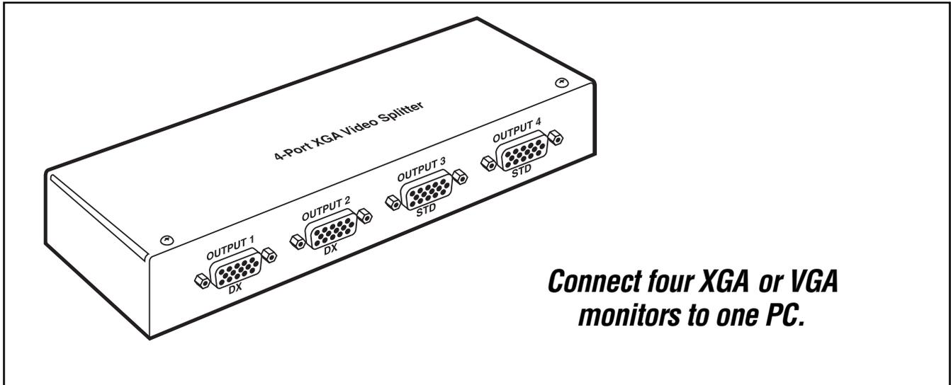
**Connect four XGA or VGA monitors to one PC.**
