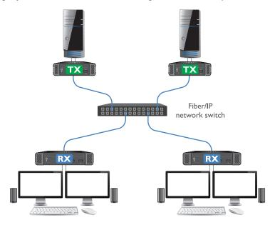
This method of connection works well for small numbers of transmitters and receivers, but will become more difficult to manage as more units are attached. The maximum number of transmitter sources that can be made available to any receiver is sixteen.
