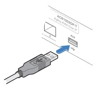
2 Connect an accompanying USB-to-serial converter to a vacant USB socket on the receiver.
