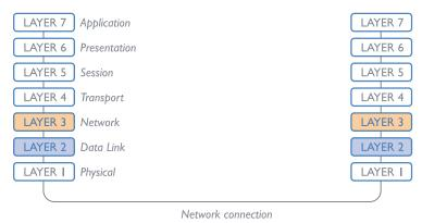
As your data travel down from you towards the transmission medium (the cable), they are successively encapsulated at each layer within a new wrapper (along with a few instructions), ready for transport. Once transmission has been made to the intended destination, the reverse occurs: Each wrapper is stripped away and the instructions examined until finally only the original data are left.
