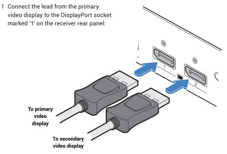
2 If required, connect the lead from the second video display to the DisplayPort socket marked '2' on the receiver rear panel.
