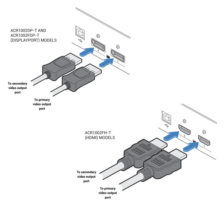
2 Connect the plug at the other end of the cable(s) to the corresponding video output socket(s) of the host computer.
