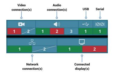
These useful status indicators will be displayed in the top left corner (or elsewhere according to UI Settings) of the primary console display:
