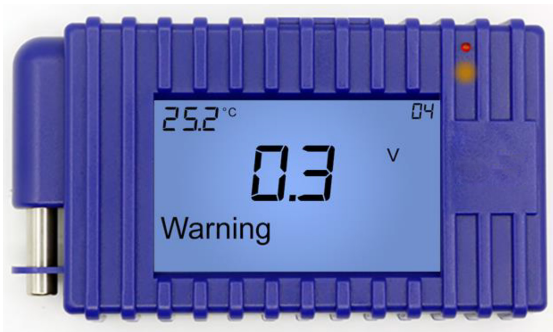
FIGURE 4-5: EXAMPLE OF SENSOR IN WARNING STATE (YELLOW LED BLINKING)
