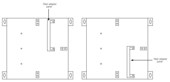
Figure 6. Position the fiber bracket on the top or bottom.
