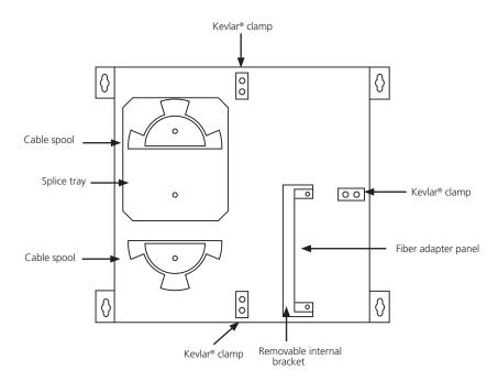
Figure 2. Inside the enclosure.
