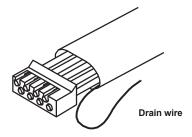
5. Push the loading bar and cable into the housing. (Make sure the loading bar fits tightly in the housing.)
